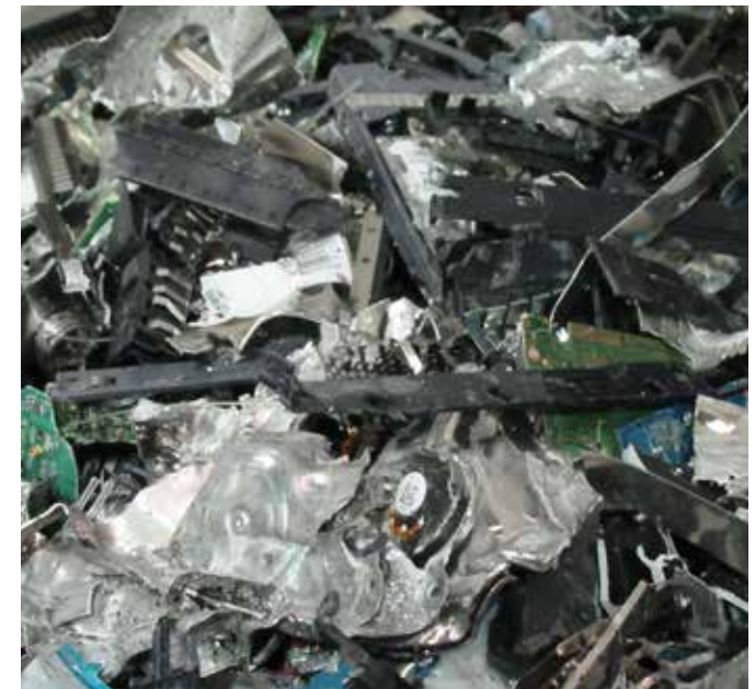
Figure 5: Hard drive destruction
